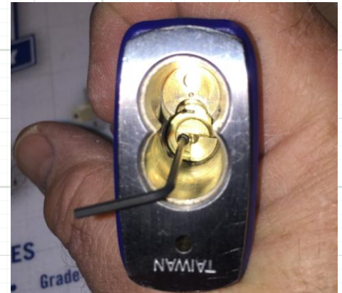
Using a 1.5mm Allen wrench, turn set screw Clockwise to open the shackle. Then turn set screw counter clockwise to remove the key retaining set screw.
